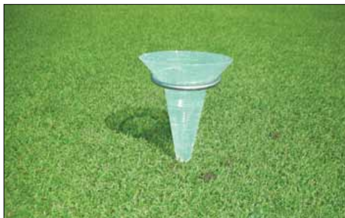
Figure D-1. Catch can with stand and measurement readings. Source: EC Design, LTD.
