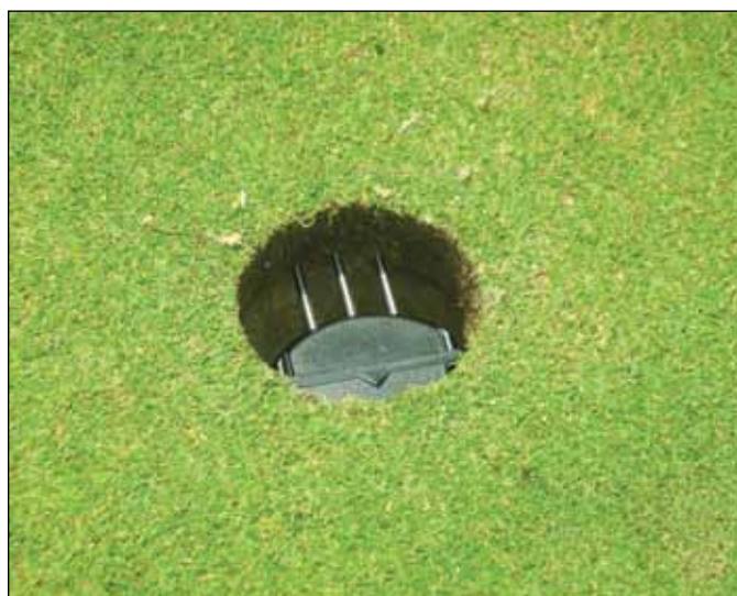
Figure 3-4. Underground wireless soil sensor providing soil profile feedback to irrigation central control. Source: EC Design Group, LTD.
