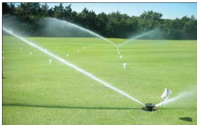
Figure D-2. Sprinkler operation during catch can test. Source: EC Design, LTD.
