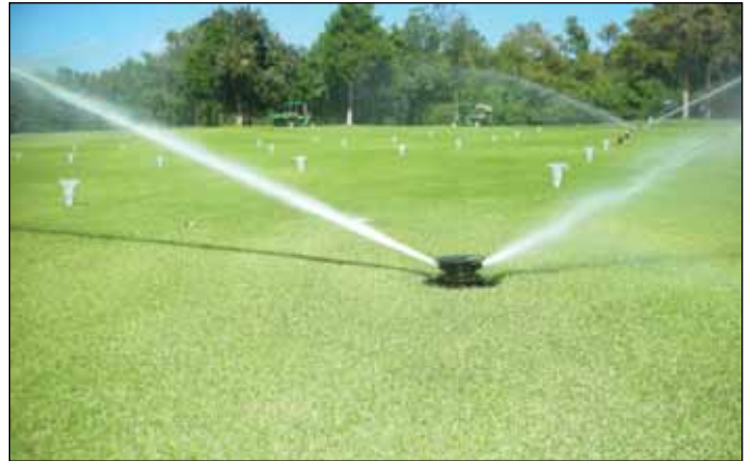
Figure 3-12. Catch can test layout in fairway. Source: EC Design Group, LTD.
